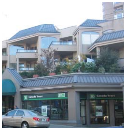
Buildings with upper floors stepped back can incorporate rooftop balconies and provide relief to the streetscape.
