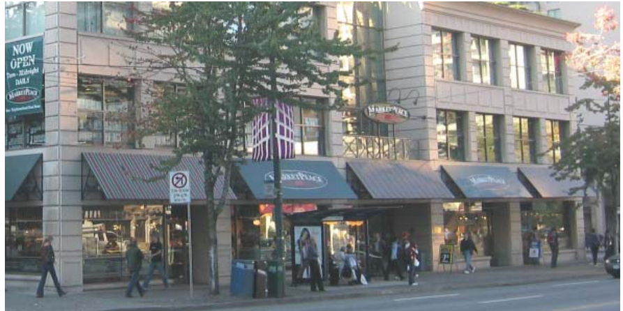
The facades of this mixed-use building (above) and residential building (below) are articulated with individual bays, each with its own window treatment or entry way.
