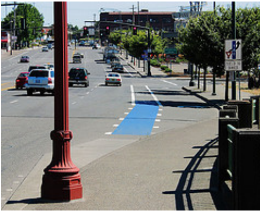
Bicycle lane treatment at a right-turn-only lane
